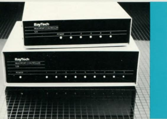
The 500D series of non-buffered printer controllers allows computers to share one or more printers without switching cables. They connect easily to RS232C serial ports on computers and printers. If configurations do not match, the printer controllers may be easily reconfigured via a menu-driven configuration mode. Configuration data is stored in non-volatile memory.
